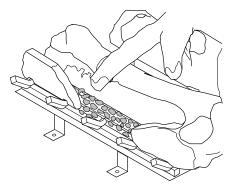
Figure 47 - Placing Ember Material on Burner
